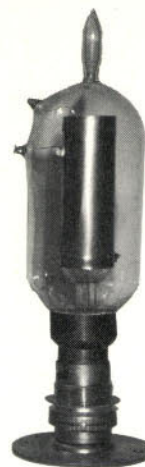
Then the valve gradually evolved... (this is a Round Type C)
