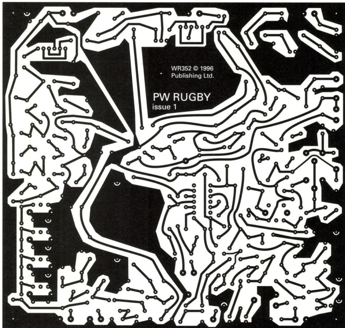
Fig. 2.2: The p.c.b. track diagram.
